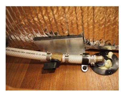
3. Make sure the valves close to the water screen are open. It is unlikely these valves will be closed.
